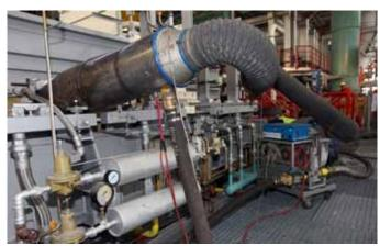
Finally the service division of HORN heats up the furnace to operation temperature with special heat-up burners and measurement equipment to ensure the proper temperature gradient and controlled expansion of all refractory material.
