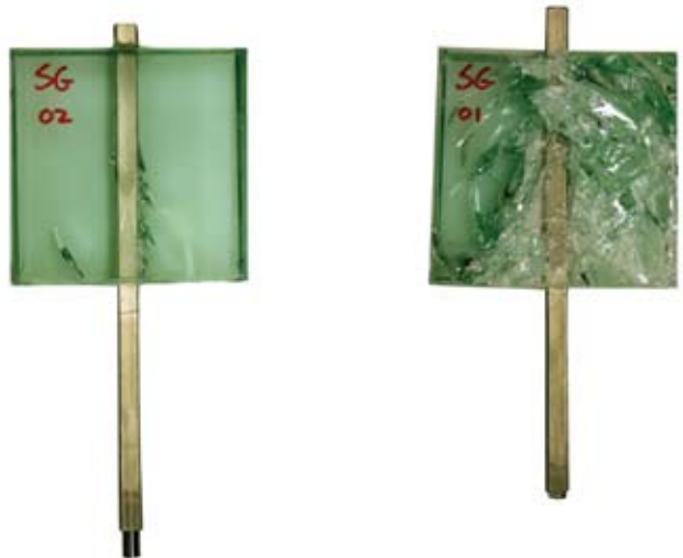
Figure 8: Specimen SG(23)#02 shows only minor cracks in the inner layer, whereas specimen SG(23)#01 shows severe cracking. Both specimens have been tested at room temperature.
