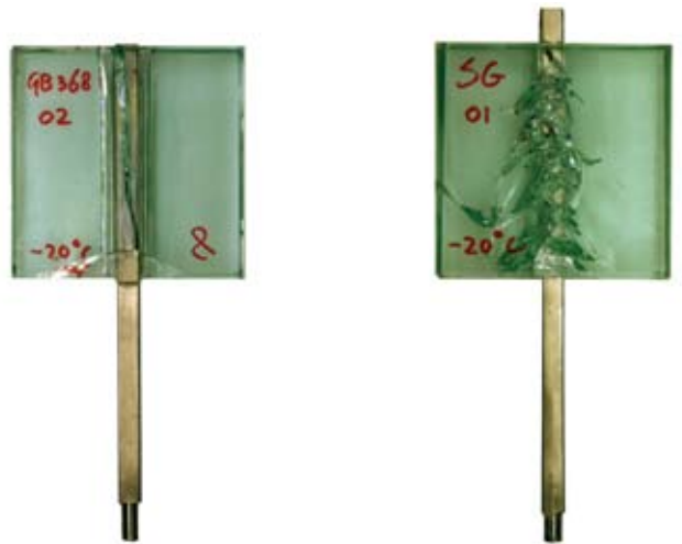
Figure 9: Specimen ACR(-20)#02 shows a linear crack (left) and specimen SG(-20)#01 shows more severe cracking.
