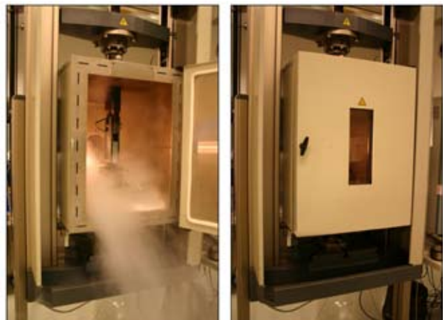
Figure 5: A climatic chamber has been put around the test setup to either cool to -20°C (left) or heat to 60°C (right).
