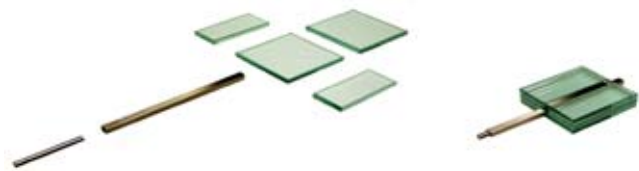
Figure 1: Exploded and assembled view of the pull-out specimens.
