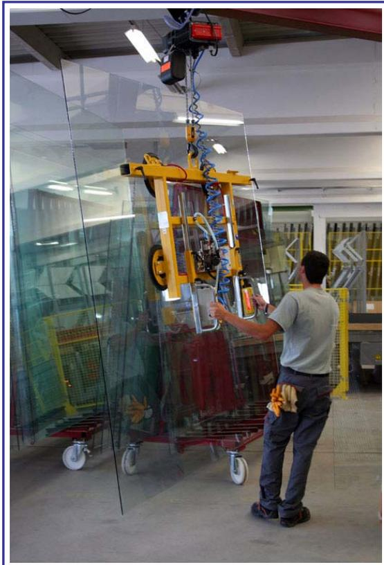
The Venturi device 7005-AB is used to supply the insulation glass unit with large glass panes; the device is used otherwise in the manual cutting unit for feeding the cutting table with glass. Depending upon design, this type of device up can transport up to 1200 kg and sized up to 6.0 x 3.2 m. The extendable side tubes help when adapting to the glass dimensions. If required, these support tubes can also manufactured in such a way that they can be removed.
