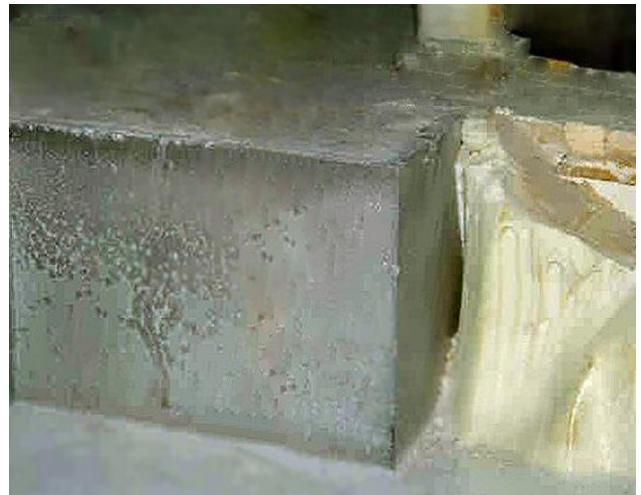
Fused cast block, fully protected by ACT ® during a two-year opal campaign
