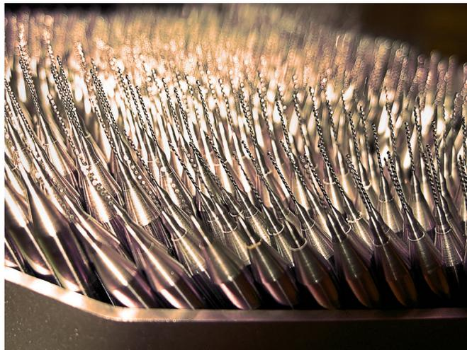
The nTRIBO process is an economical and flexible batch process capable of coating thousands of objects (drills, wire guides, nozzles etc.) in single batch. Beneq provides a turnkey solution with the nTRIBO coating system TFS 500.
