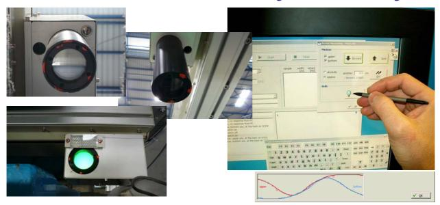
Stresstter  $6^{\text{TM}}$  is a modern machine for automatic off-line non-contact and non-destructive stress measuring in the sheet glass. Stress is measured in several spots across the width of the sheet. Measured stress vector has the orientation of the flowing glass on the production line. Stresstter  $6^{\text{TM}}$  is designed to operate with sheet glass of these parameters: length of 1200 to 6000 mm, thickness of 1.6 to 20 mm and width of 1200 to 5600 mm.
