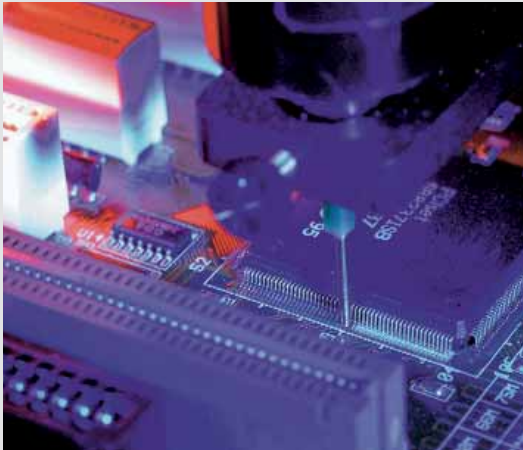
Fixing of soldered contacts of electronic components
