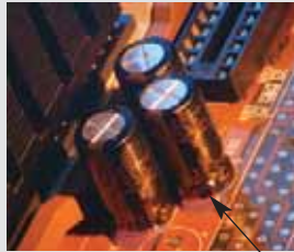
Protection against vibration of soldered electronic components
