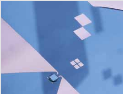
Smart inlay – flip-chip bonding
