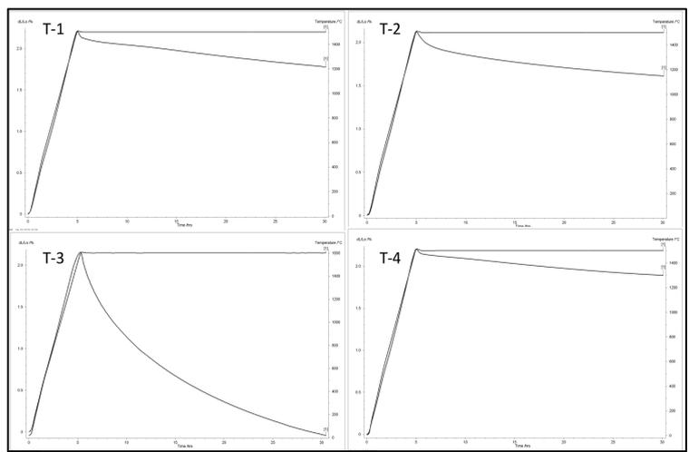
**Figure 4:** Creep Curves for T-1 to T-4
