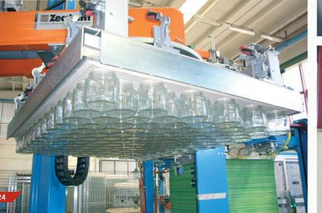
Palletizing column and pickup head supporting arm
