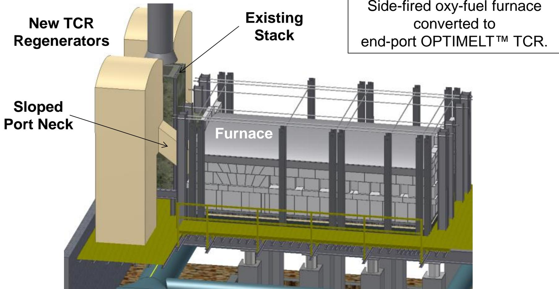
Furnace can be operated with and without OPTIMELT™
