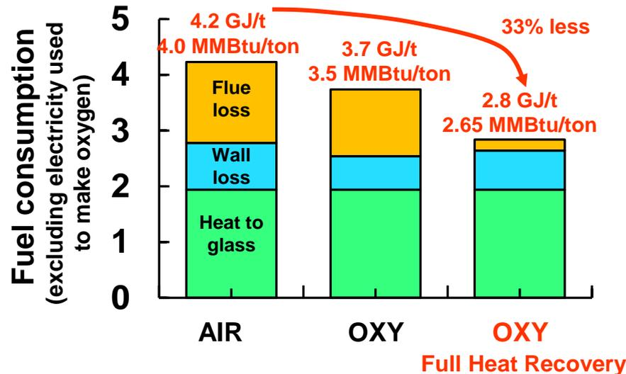
Significant Heat Available for Recovery in Oxy-fuel Flue Gas
